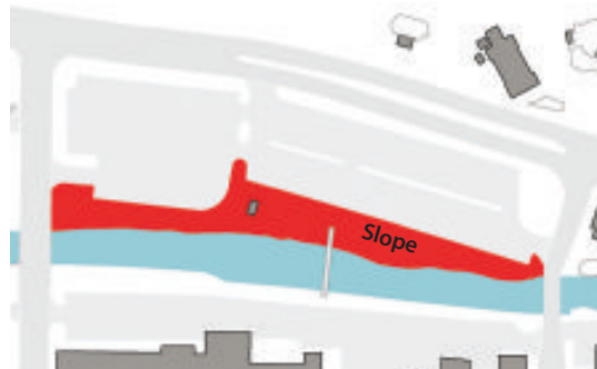
Figure 35: Slopes. The banks of the river here are relatively steeply sloped. Vegetation should be maintained to help stabilize the bank, and stormwater should not be allowed to run freely down the slope.
