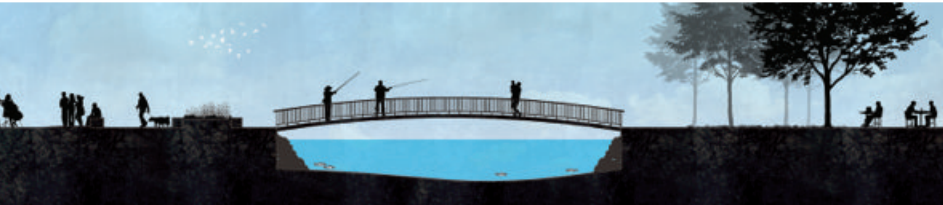
Illustration 27: Pine Street Pedestrian Bridge Section. The proposed bridge acts as a gateway into the Warehouse District, connecting the bustling downtown with this up-and-coming part of town. The bridge has been designed to be 12 feet wide, to accommodate free flow of foot traffic and allow fishing.
