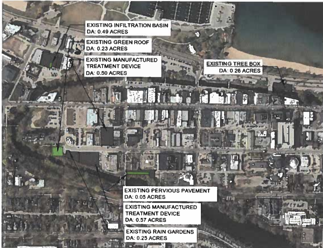
Figure 45. Existing BMPs Identified During Field Investigation
