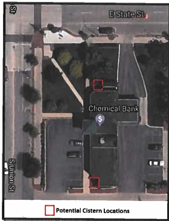
Figure 68. Potential Cistern Locations on Chemical Bank Site
